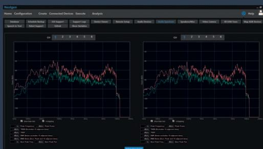
ATAM Audio Analysis showing real time FFT audio spectrum, Total Harmonic Distortion and Signal to Noise calculation. Data can be utilised during automated testing to ensure audio quality and check for signal issues such as noise, distortion and dropouts.
