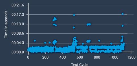
Analysis of Bluetooth Reconnection performance used by an automotive OEM to optimise new firmware build. Bluetooth reconnection time over 1000 cycles showing connection time variances.
